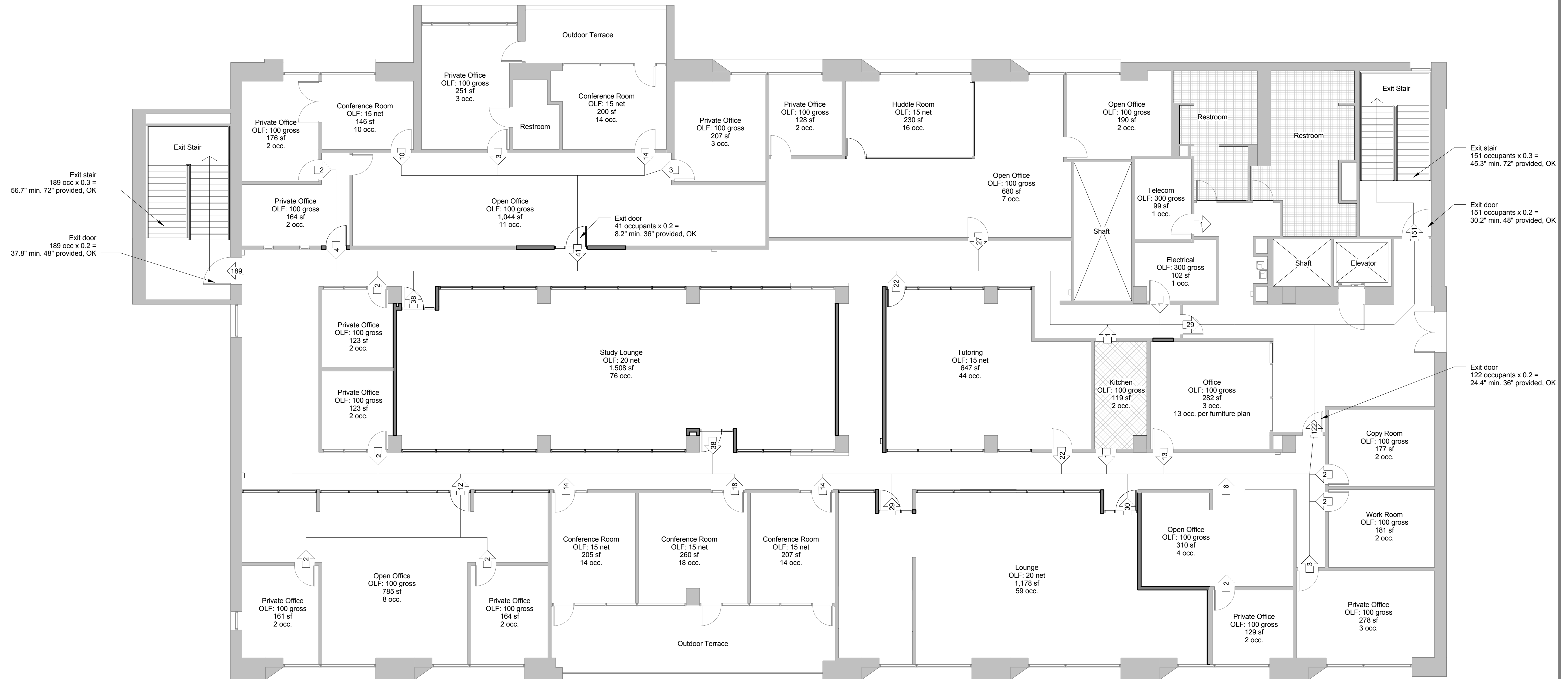
③ First Floor Code Plan (East Stair) 1/8" = 1'-0"
