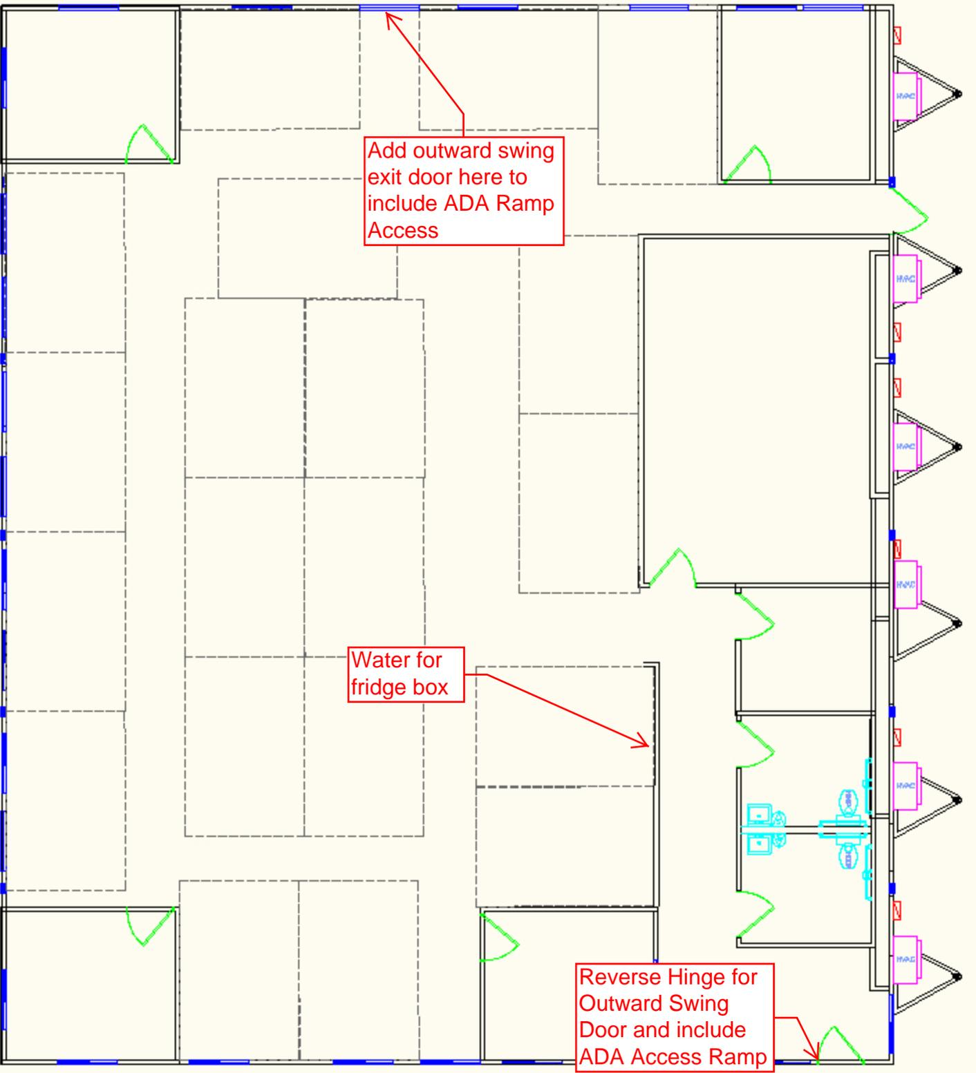
Add outward swing exit door here to include ADA Ramp Access
